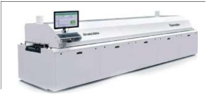
VITRONICS SOLTEC Centurion 12 thermal zones. N2 ready
