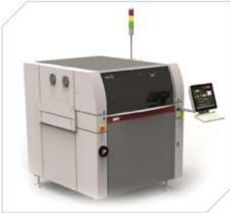
DEK NeoHorizon 3iX Printing accuracy at 2.0 Cpk @ +/- 25 µm
